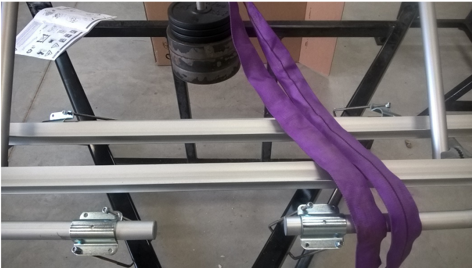
Photo 4, situation after mechanical pull side wards (under 50 kg load).
